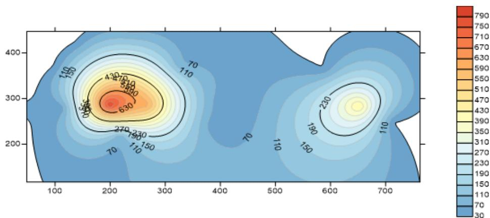
Figure 7. The schematic map of the exposure dose of tailing № 5 (μR/hour).
